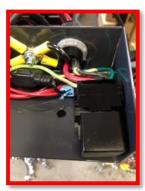
3. Inline fuse. Found inside electrical box. (7.5amp automotive type 2 prong fuse) <u>https://www.youtube.com/watch?v=JZZmYQtybAE</u> replacing fuse
