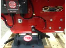
**Step 9** – Adjust the machines tilt by loosening the two black adjustment levers on the base of the machine. There is one at the front and one at the rear of the 300E & 400E machines, it is an optional feature on the 200E machine. Tilt the machine to the desired angle and then retighten both adjustment levers. The angle of the levers can be moved by pulling the lever out and rotating it to the desired position.
