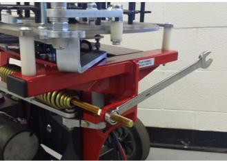
**Step 15** – The pull cord or optional radio release can now be connected to the machine. Pull cord will connect through the yellow- ended cord.
